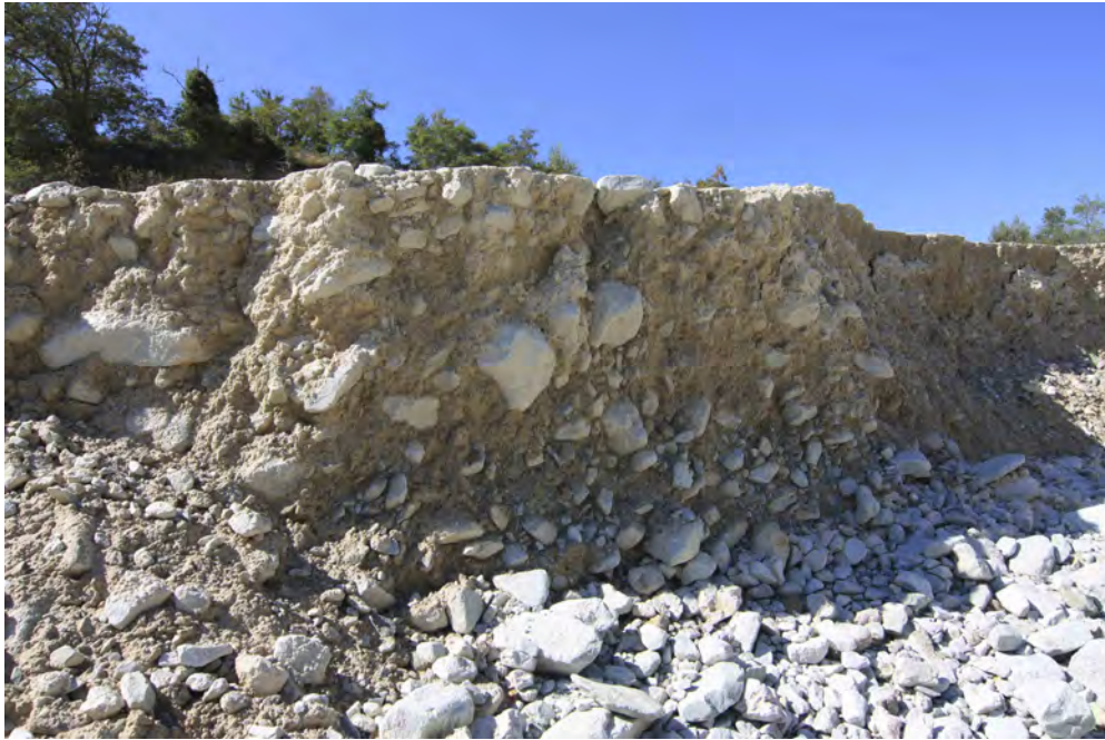
Figure 2.8: Visual impression of the debris flow material. The picture was taken after the debris flow event on 09.08.2009 right at the confluence of the Illgraben and the Rhone River.
