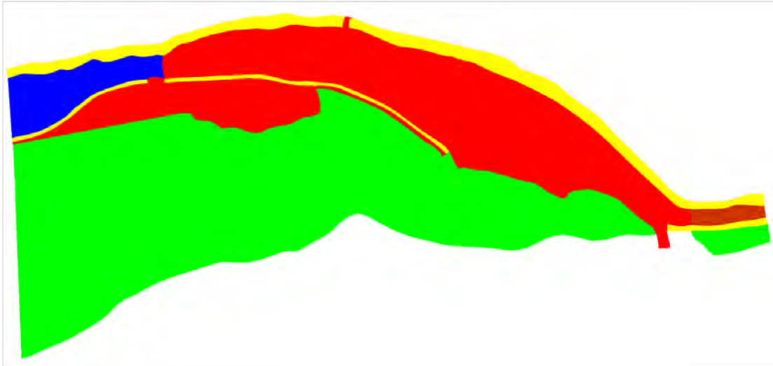
Figure 4.10: Subdivision of the 2D model domain into five different areas (brown: bed1, red: bed2, blue: bed3, yellow: embankments, green: floodplain).
