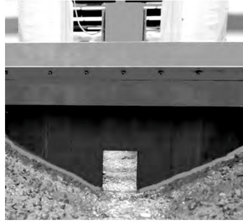
Figure 4.4 – A picture of the channel with constriction composed of multiple PVC elements (view from upstream to downstream).
