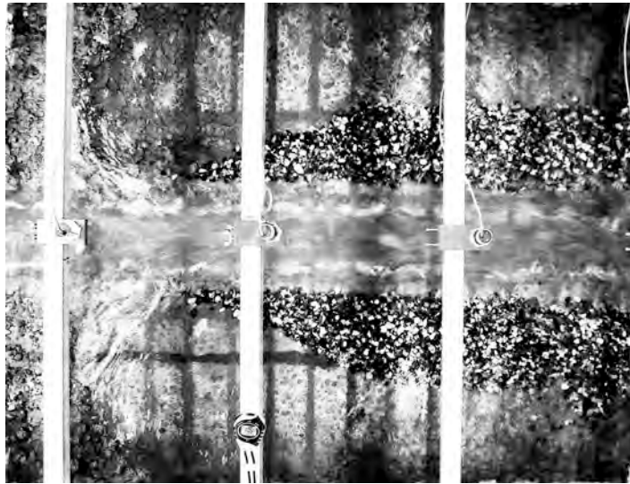
Figure 7.12 – The remaining sediment deposits at the end of the hydrograph test Hy-o.
