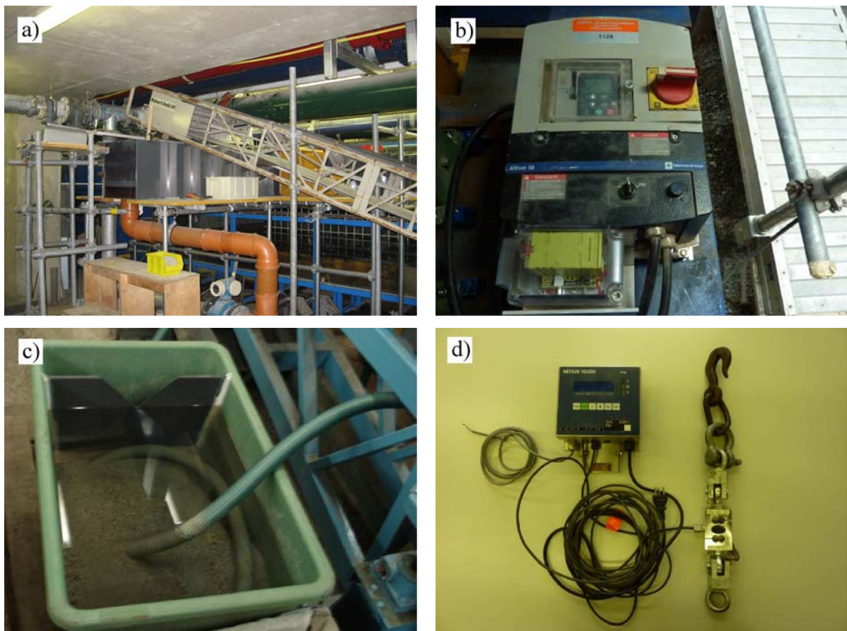
Figure 3-21: Instrumentation for sediment management during the experiments. a) Conveyor belt for the sediment feed, b) Velocity regulator for the conveyor belt. c) Sediment trap for removing the transported sediments. d) Scale used for the control of the sediment balance.
