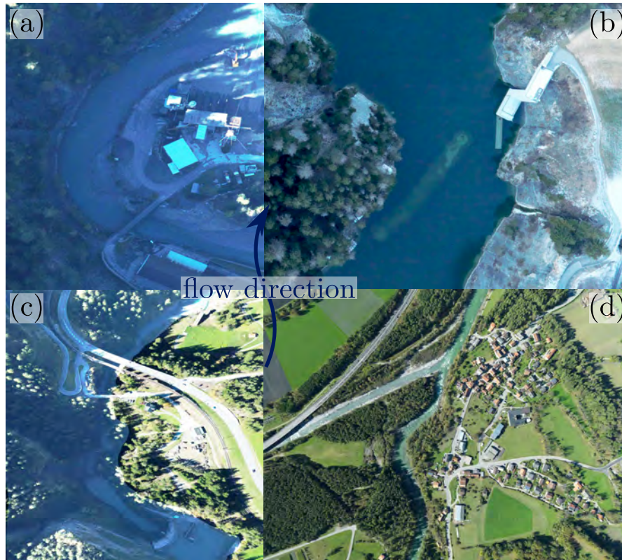
Figure 3.4: Aerial pictures representing: (a) gravel quarry at the upstream end of the reservoir, (b) intake structure of Solis SBT with submerged guiding structure in the reservoir, (c) Solis Dam and SBT outlet structure, and (d) confluence of the Albula to the Hinterrhine.
