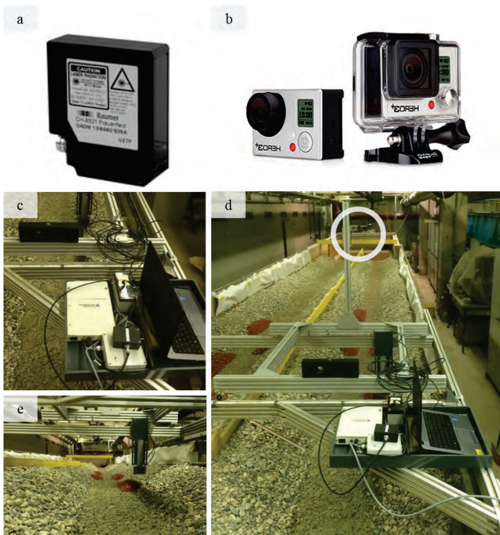
Figure 3.7 – (a) Laser scanner, (b) camera: GoPro Hero 3+, (c) acquisition system, (d) moveable instrumentation installed on carriage and (e) laser scanner on the support
