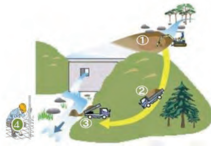
Figure 2.7 – Schematic representation of replenishment of sediment method, from the excavation point to the delivery of material on the river (in Kantoush et al. (2010b))
