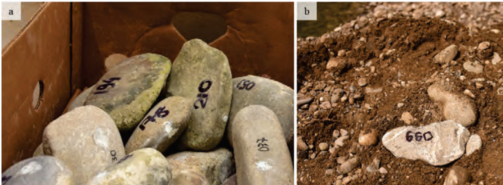
Figure 9.5 – (a) Traced gravels and (b) numbered stone with RFID tag placed on one deposit
