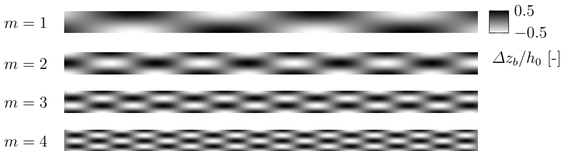
Fig. 3.13.: Sketch of free bar topography for different lateral modes m
