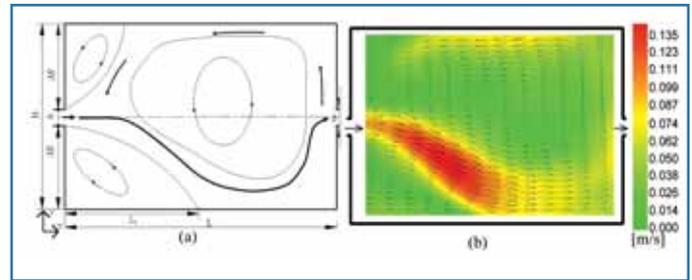
Figure 5. (a) Time averaged flow pattern and velocity magnitude (m/s) for clear water obtained by LSPIV measurements, (b) Plan view of the reference experimental setup ( $L = 6$  m,  $B = 4$  m) and definition of the geometrical parameter of the first recirculation cell in the basin ( $L_r$ ). Discharge  $Q = 7,0$  l/s, and water depth  $h = 0,2$  m.
