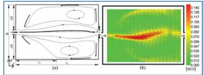
Figure 6. (a) Time averaged flow pattern and velocity magnitude (m/s) with sediment entrainment flow obtained by LSPIV measurements after 4,5 hours, (b) Plan view of the reference experimental setup ( $L = 6$  m,  $B = 4$  m). Discharge  $Q = 7,0$  l/s, water depth  $h = 0,2$  m, and suspended sediment concentration  $C = 3,0$  g/l.
