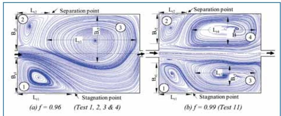
**Figure 2. Time-averaged streamlines obtained by LSPIV measurements for clear water flow for two different basin geometries with shapes  $f = (A/P^2) * ER$  of 0,96 (left) and 0,99 (right). The geometrical parameters of the recirculation cells in the basin are  $L_{ri}$ ,  $B_{ri}$  for gyres (1, 2, 3 & 4).**
