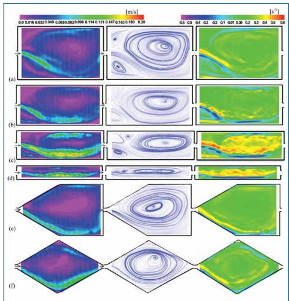
Figure 3. Average flow pattern with velocity vectors (left), streamlines (middle) and mean vorticity (right) for five different geometries with shape factors  $f = 0,96$  (a),  $0,67$  (b),  $0,375$  (c),  $0,122$  (d),  $0,75$  (e), and  $0,95$  (f). Without sediments.
