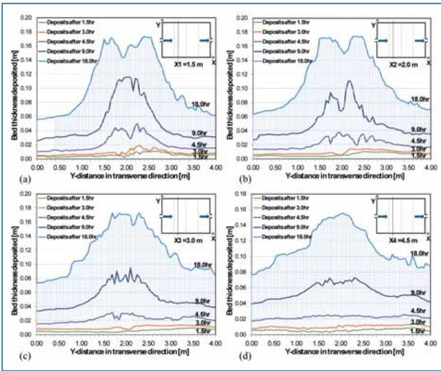
Figure 8. Comparison of bed profiles at different cross sections of the basin, (a)  $X1 = 1,5$  m, (b)  $X2 = 2,0$  m, (c)  $X3 = 3,0$  m and (d)  $X4 = 4,5$  for runs (2, 3, 4 and 5), after (1,5, 3,0, 4,5, 9,0, and 18 hours). Water depth  $h = 0,2$  m.
