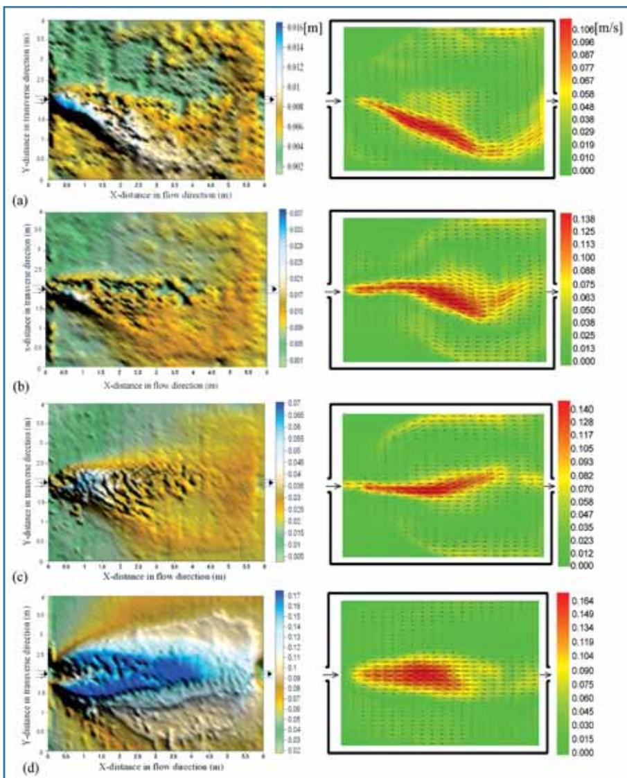
Figure 7. Long-term morphological evolution of deposition in m, (left) and flow patterns and velocities in m/s, (right) after different runs time steps (a) after 1,5hr, (b) after 3hr, (c) after 4,5hr (d) after 18,0hr. Discharge  $Q = 7,0\text{ l/s}$ , water depth  $h = 0,2\text{ m}$  and suspended sediment concentration  $C = 3,0\text{ g/l}$ . Caution: Full scale changes in each case.
