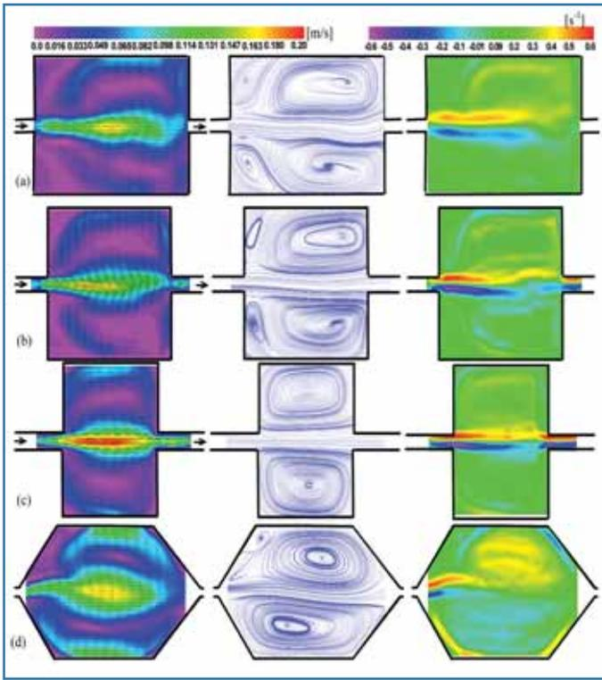
Figure 4. Average flow pattern with velocity vectors (left), streamlines (middle) and mean vorticity (right) for four different geometries with shape factors  $f = 0,97$  (a),  $0,98$  (b),  $0,99$  (c), and  $1,71$  (d). Without sediments.
